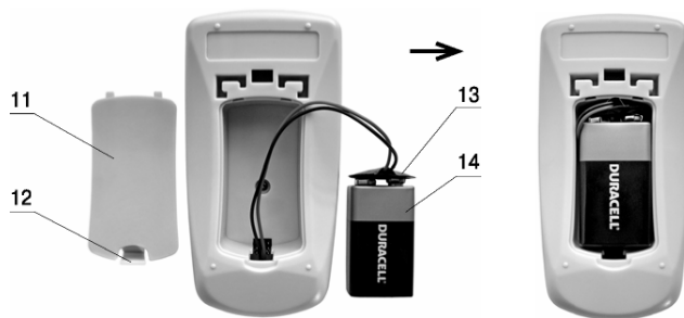
Figure 2 – Power battery mounting
